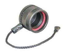
Watertight aluminum alloy cover protects CB Series plugs from damage when unmated. Black zinc plated. O-ring holds cover in place. Supplied with nylon rope, with ring terminal or loop. Attach with ring terminal, or attach to cable with loop. Maximum weight 7 grams.
