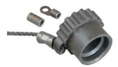
Black nitrile rubber cover fits all CB Series receptacles including shrouded versions. Tight friction fit prevents water ingress to unmated connector. Supplied with nylon rope, ring terminal and ferrule. Terminal and ferrule are supplied unassembled. Attach to panel with ring terminal, or attach to cable with crimp ferrule. Use standard crimp tools for installation. Maximum weight 5 grams.
