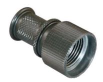
Black zinc plated aluminum alloy adapter fits all CB plugs and receptacles with M14 x 1 threads. Attach adapter to connector and fill with potting compound for wire protection and waterproofing. Attach shield and cable strength members to adapter with Glenair tool 600-061 using 3mm stainless steel **BAND-IT**® straps. Maximum weight 7 grams.
