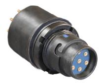
Eliminate unwanted high frequency electrical interference with European standard filtered CB07 connector. Stainless steel body and jam nut, with black chrome finish. Mates to standard CB07 plug connectors. Printed circuit board contacts are gold plated. Watertight when unmated, CB07 filtered connectors offer 5000 cycles of mating and meet harsh environment requirements.
