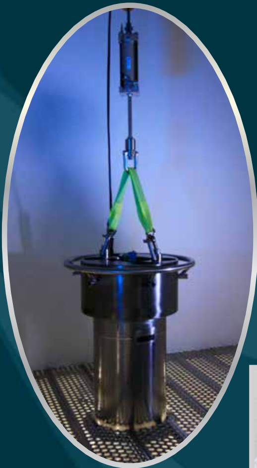
LARGE PRESSURE VESSELS: Built to accommodate complete cable assemblies, mated connectors, and customer-supplied sub-assemblies. Each unit contains a 12" diameter X 72" depth test chamber accommodating specimen weights up to 1500 lbs.
