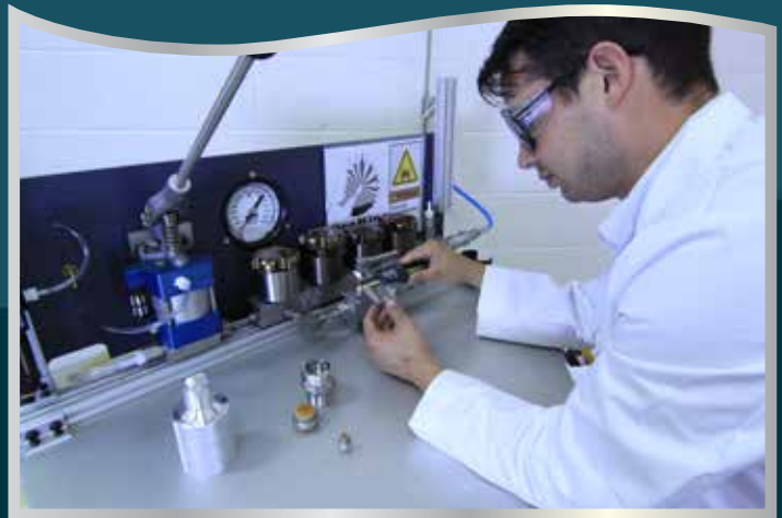
DISCRETE CONNECTOR TESTING: All Glenair subsea interconnects are subjected to 100% inspection and test
