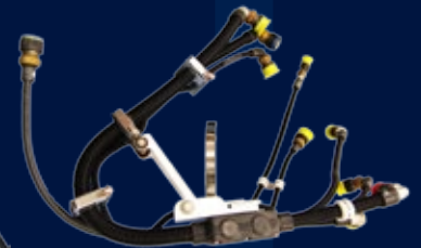
Aircraft wheel well / landing gear wired conduit assembly
