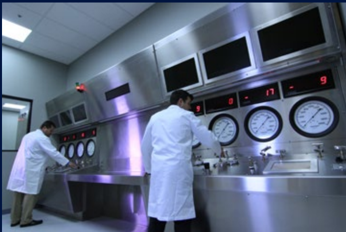
Glenair's hydrostatic test lab control room: modular consoles provide for up to 8 pressure circuits, operating in manual or automated mode. Each circuit is capable of a maximum of 16.5K psi.
