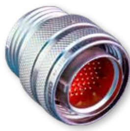
High-reliability connector savers prevent mating cycle damage to receptacle connectors during qualification and test, significantly reducing wear and the possibility of damage prior to delivery
