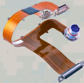
Integrated Flex / Rigid Flex Circuit Assemblies
