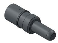
Series 927-072 contacts for size #16s through size #0 wire. Copper alloy with silver or gold plating, terminate to wire with standard crimp tools. Contacts are front-release. Use in series 927-072 connectors.
