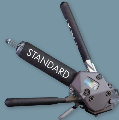
BandMaster™ ATS EMI/RFI Shield Termination System
