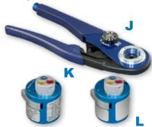
Crimp tool for use with size #20, #16 and #12 power pins. 9.75 inches OAL, 1.25 pounds. Use with M39029/57 and /58 contacts and 809-093 adapters.
