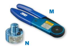
For crimping size #16 shield sleeves. These mil spec approved tools feature a ratchet mechanism to prevent damage from over crimping. Check calibration with M22520/3 gage.
