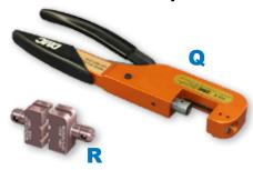
Parallel action tool for use with hex crimp dies. 11 inches OAL, 2.0 pounds. Anodized aluminum frame, steel mechanism, plastic handles. Includes tool for die set extraction. Accepts all M22520/5 die sets.
