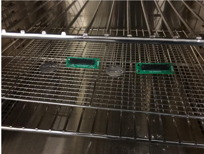
Figure 24: Samples 2A and 2B ready for Humidity Exposure Testing
