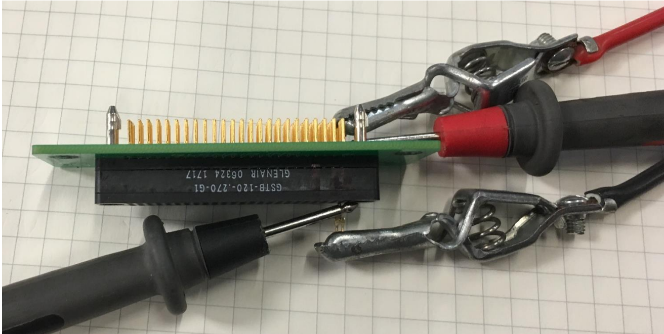
Figure 12: Stacker Connector Sample during Low Level Resistance Testing
