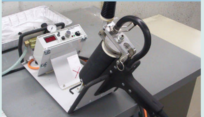
▼ Original hot melt overmolding tool (furnished to the Glendale factory by Glenair UK).
