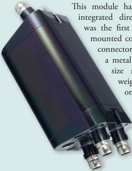
▲ An early example of a “braze-on” hub, made in 2009, with the Mighty Mouse panel plugs integrated directly into the box.
