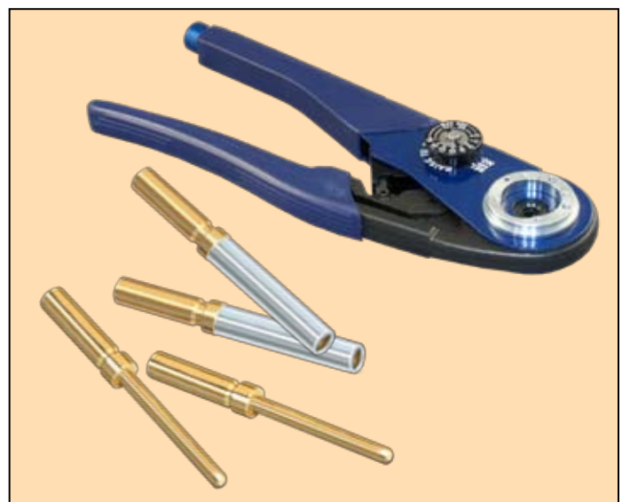
High-Performance Series 80 “Mighty Mouse” #23 gage crimp contacts are made from beryllium copper alloy and gold-plated per ASTM B488 Type 3, Code C.
