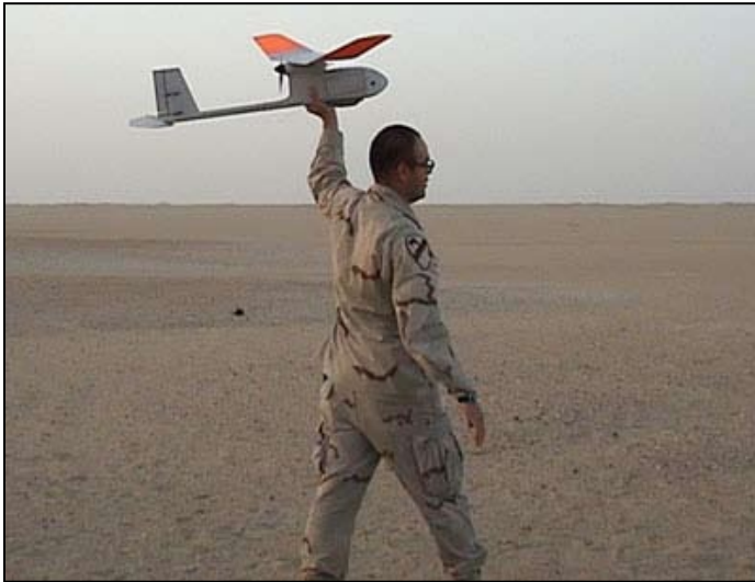
The most advanced small UAV deployed with the U.S. Armed Forces, the AeroVironment Raven can be operated manually or programmed for autonomous operation.
