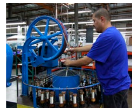
Glenair can also offer AmberStrand® users direct factory overbraiding services for both point-to-point as well as multi-branch interconnect assemblies.
