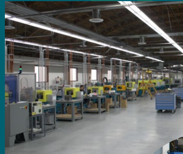
Just a small portion of Glenair's composite thermoplastic injection molding equipment used in the fabrication of lightweight, corrosion-resistant connectors and backshells
