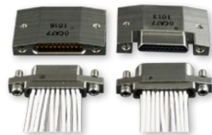
▲ Well-Master® 260° connectors withstand temperatures to 260°C and feature unique angled mounting ears for incorporation into cylindrical packages such as those found in downhole tools
