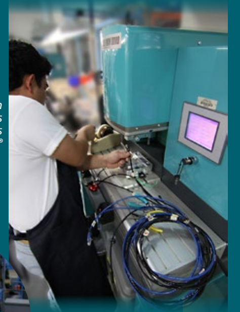
Just a small portion of Glenair's composite thermoplastic injection molding equipment used in the fabrication of lightweight, corrosion-resistant connectors and backshells
