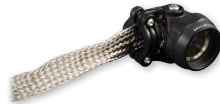
▲ The Swing-Arm™ is a unique 3-in-1 backshell that provides straight, 45°, or 90° cable routing—all in one part; reducing BOM part number proliferation. The version above integrates a lightweight metal-clad composite braid sock for reliable shield termination.
