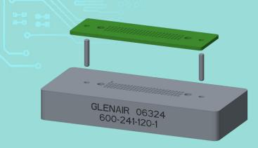
2. Place the board on the support plate and align board clearance holes with the guide pins.
