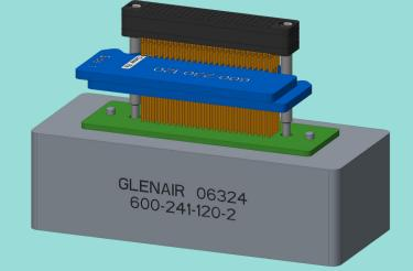
4. Remove the combs and slide the connector pins into the mounting plate.
