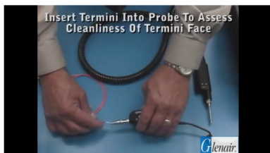
Fiber Optic Terminus Cleaning and Testing - Step 6
