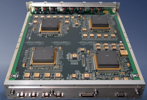
Physical layer SpaceWire router aboard the James Webb Space Telescope (NASA)
