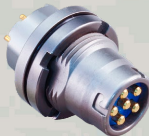
Filtered radio-mount jam nut audio receptacle with non-rigid spring contacts, solder cup or PC tails
