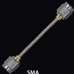
SMA 086 cable, tinned-copper braid DC-18 GHz
