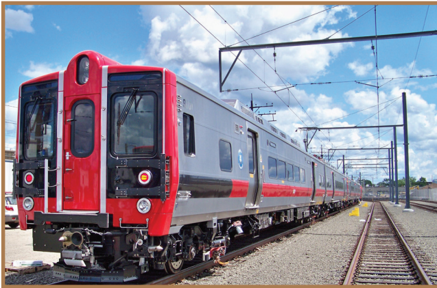
The M8 is an electric multiple unit (EMU) railroad car built by Kawasaki for use on the New Haven Line of the Metro-North Railroad. Photo: office of Dannel Malloy
