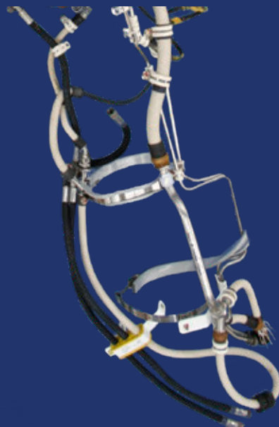
Metal-core conduit wire protection aircraft brake assembly
