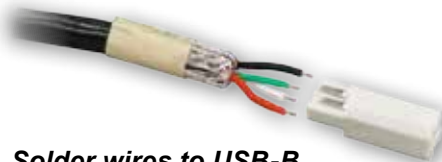
Solder wires to USB-B Insert
