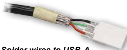
Solder wires to USB-A Insert
