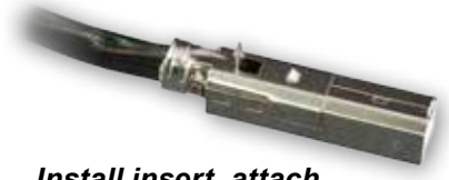
Install insert, attach lid, and crimp shield
