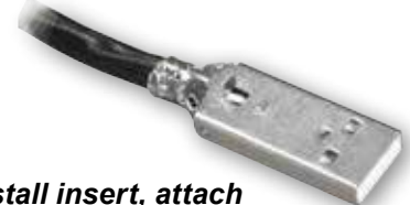
Install insert, attach lid, and crimp shield
