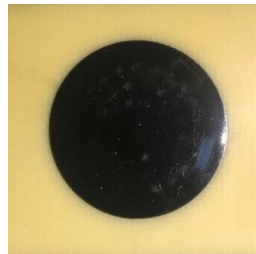
Reinforced solder joint with potting
