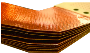
Multilayer rigid-flex circuit assemblies—up to 27 layers—offer increased circuit density while still maintaining the medium's dynamic 3D flex characteristics
