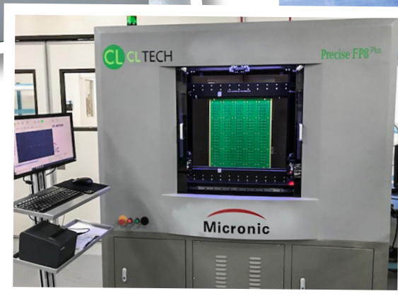
Automated Optical Inspection and Flying Probe Electrical Test
