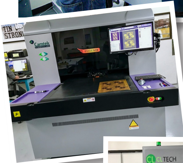
Automated Optical Inspection and Flying Probe Electrical Test
