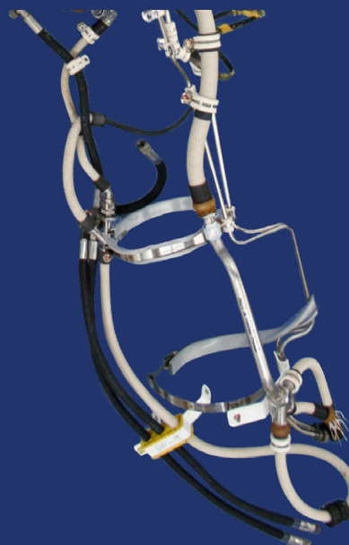
Metal-core conduit wire protection aircraft brake assembly
