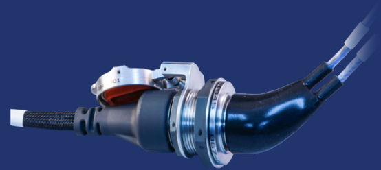
Mated GateLink Pro™ plug and receptacle cordsets with shielded twisted pair cabling. Plug side features environmental overmolding, receptacles side utilizes strain relief boot
