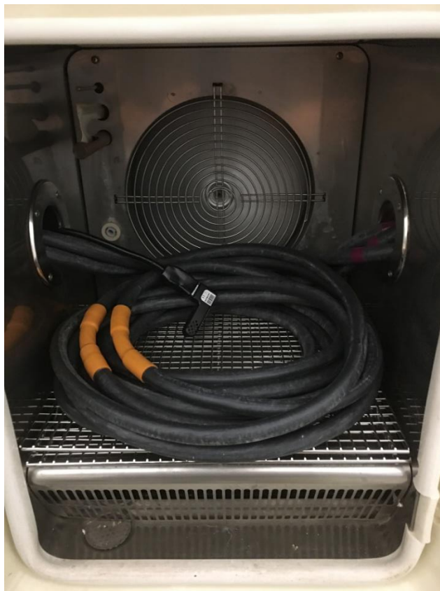
Image 6 : Curing of Autoshrink samples with Glenair Duraelectric adhesive, +40C @ 50% RH for 48 hours.
