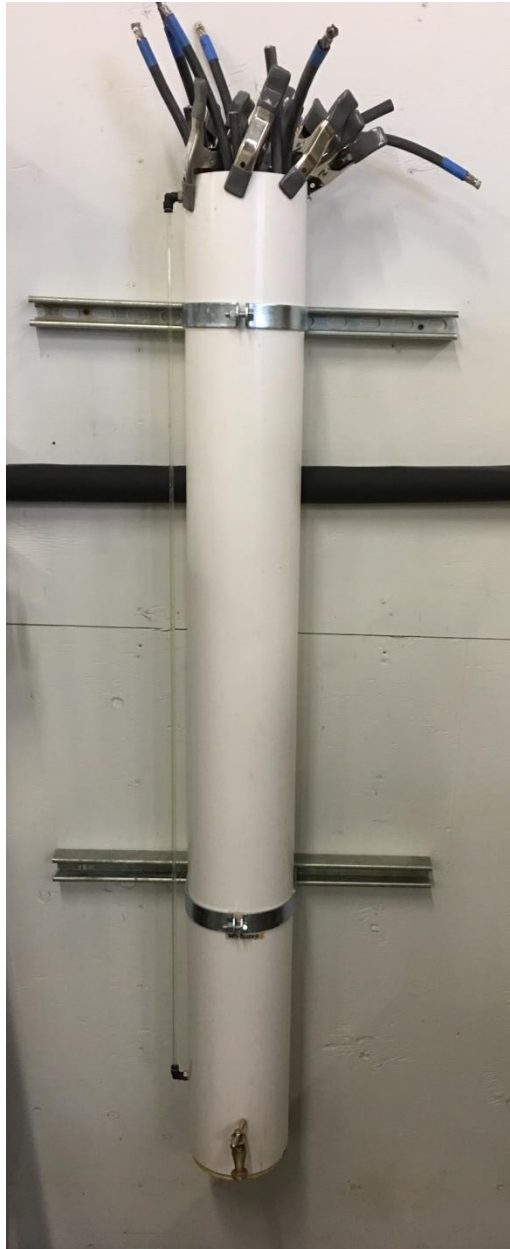
Image 2: Immersion insulation resistance tank.
