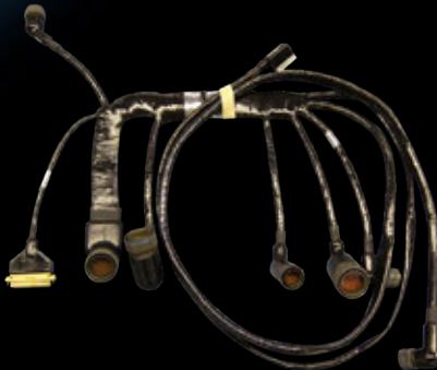
Multibranch interconnect cable harnesses and assemblies—terminated, tested, and ready for use
