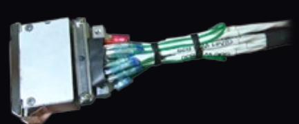
Example rectangular interconnect assembly outfitted with heat shrink termination grounds
