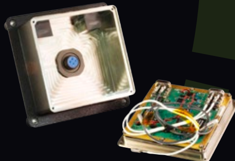
Small form-factor opto-electronic media converter with field fault monitoring
