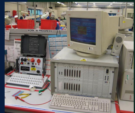
Glenair UK operates an independently accredited BS9000:CECC:IECQ test lab for both internal as well as third-party product development / design verification and connector qualification
