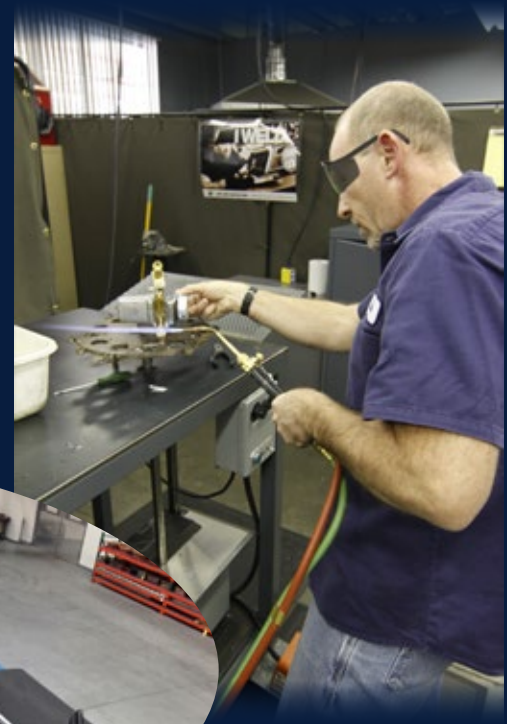
Many specialty interconnect components such as 45° and 90° angled backshells require skilled welding and/or brazing.
