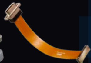
AlphaLink® board-level pogo-pin connectors and flex jumpers
