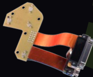
Stacked Micro-D I/O connectors with flex jumper to rigid PCB assembly
