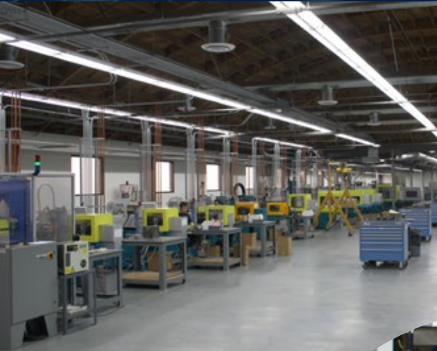
Just a small portion of Glenair's composite thermoplastic injection molding equipment used in the fabrication of lightweight, corrosion-resistant connectors and backshells
