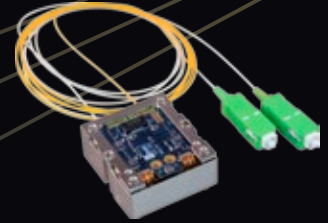
PCBA design for radio frequency-over-fiber links for SATCOM and RF signal distribution
