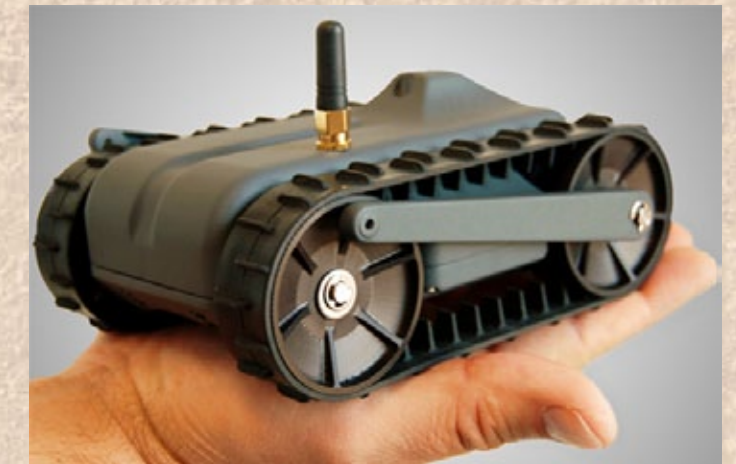
Extremely small UGVs are good examples of systems that require design attention to every aspect, including the size and weight of printed circuit boards, connectors and enclosures.
