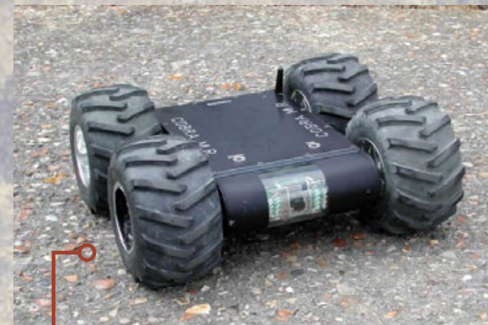
The ECA Inbot is controlled with a PDA or tablet PC and joystick. It is equipped with up to two hours of battery life and a ± 90° rotary head with color day/night as well as infrared video.
