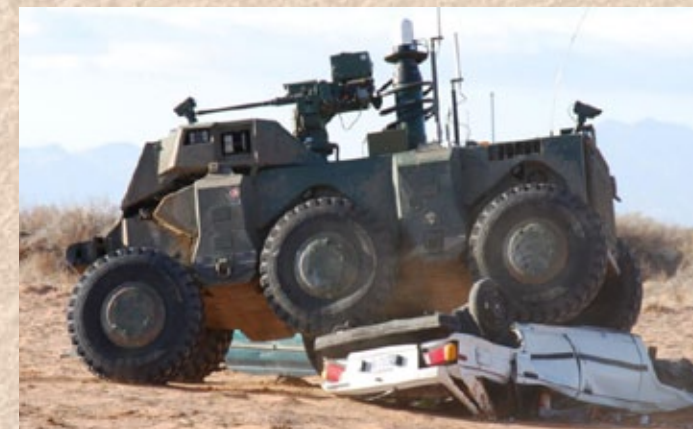
The Crusher is a 6,000 kg autonomous off-road UGV developed by Carnegie-Mellon University's National Robotics Engineering Center for DARPA. Optimized for rough terrain, the Crusher can easily overcome vertical walls, wooded slopes, and rocky creekbeds and carry 3,600 kg of armor and cargo.
