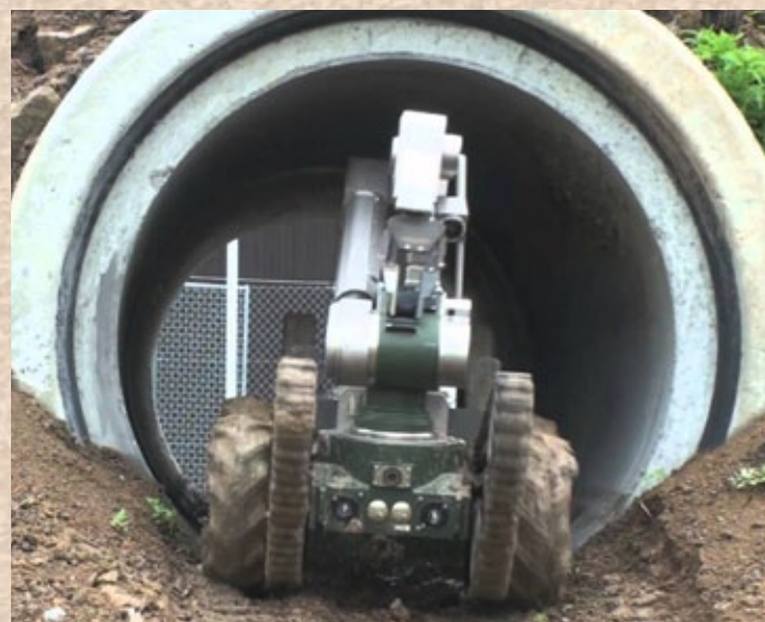
Going where soldiers don't want to go: the Cobham Telex UGV is designed for use in confined spaces and/or overcoming tall obstacles and varied terrain.
