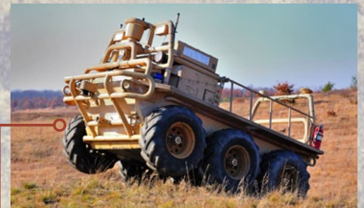
Lockheed-Martin Squad Mission Support System (SMSS), designed for transport and logistics support, is the largest UGV ever deployed with US forces.
