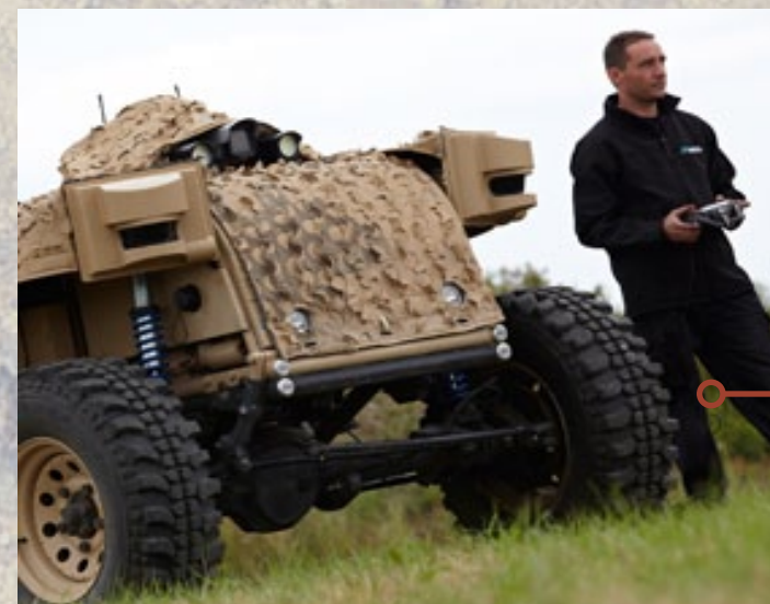
The Mira MACE 2 (Mira Autonomous Control Equipment 2) is designed for load carriage, IED disposal, casualty evacuation and perimeter control. The autonomous controlled vehicle is equipped with a land rover caliber power train and transmission to enhance speed and load-carrying capacity.
