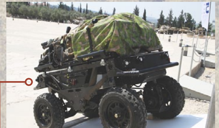
The IAI Rex Field Porter is an autonomous "follow me" vehicle, designed to support infantry units with up to 400 pounds of equipment and supplies.
