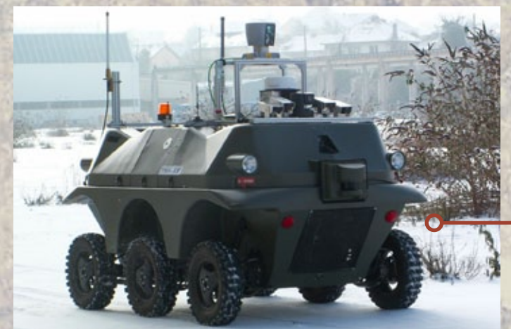
The Thales R-Trooper is a 6X6 wheeled, multipurpose UGV designed for area control, perimeter surveillance, and IED clearance, and can transport multiple small UGVs.
