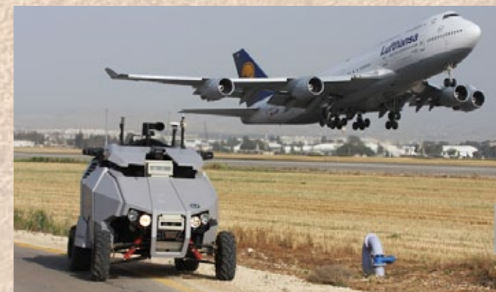
The G-NIUS Guardian MK1 is designed for routine programmed patrols and autonomous reaction to unscheduled events.
