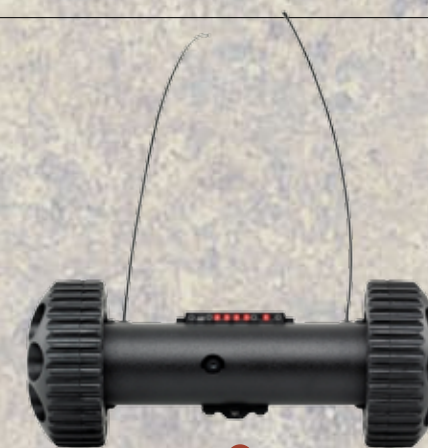
ReconRobotics Recon Scout IR tactical robot designed for tactical and SWAT applications, the man-packable and throwable MUGV is equipped with thermal/IR imaging and video broadcast capability.
