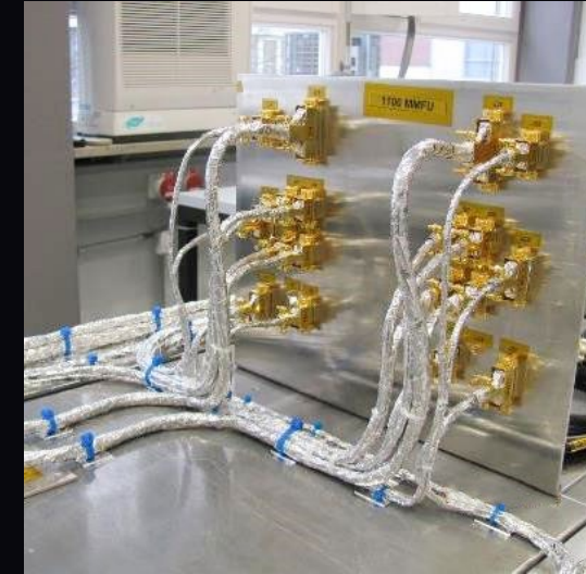
Example of ground support flat set harnessing used in developmental stages of satellite modeling, mockup, test, and mission simulation. Glenair Space Systems manages the entire process, from test cable design and fabrication to mockup integration.
