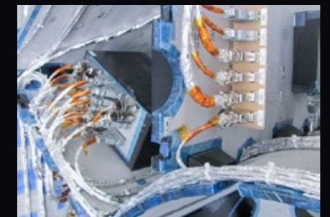
Cleanroom integration of shielded harnesses into satellite test racks
