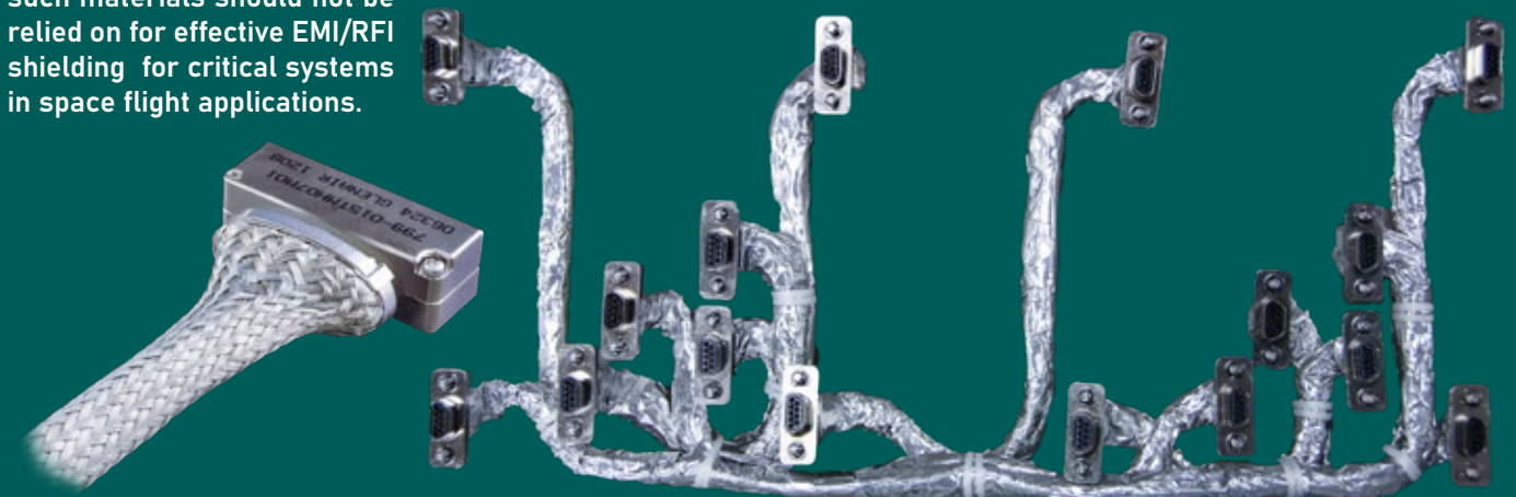
Flexible braided shielding (left) is far less likely to develop gaps and apertures that can lead to entry/exit points for electromagnetic interference as compared to foil-wrapped assemblies
