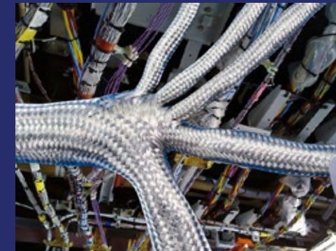
ArmorLite may be overbraided at the factory directly to multibranch assemblies, or supplied in a tubular format for on-site installation.
