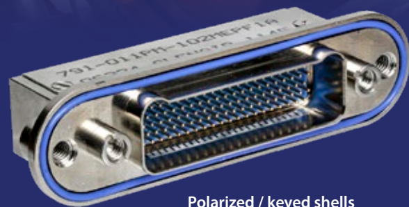
Polarized / keyed shells prevent mis-mating and allow designers to specify identical layouts side-by-side without risk of circuit damage
