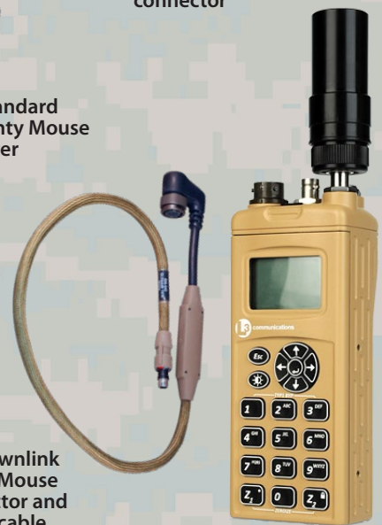
Inventus Lithium Ion conformal battery with plug-and-play Mighty Mouse 807 receptacle connector
