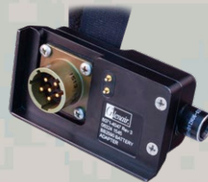
BB-2590 /BA-5590 standard soldier battery with Mighty Mouse 807 power adapter
