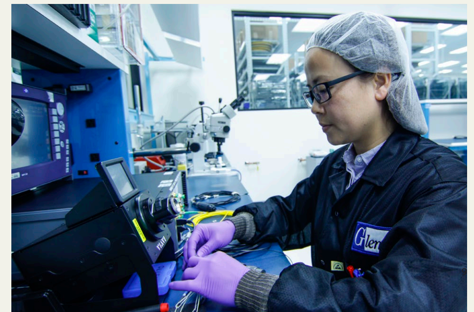
CONTROL OF ELECTROSTATIC DISCHARGE: Optoelectronic and other embedded systems are produced in special clean room facilities equipped with ESD flooring and grounding technologies.
