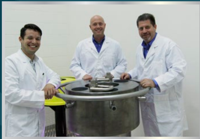
LARGE PRESSURE VESSELS: Built to accommodate complete cable assemblies, mated connectors, and customer-supplied sub-assemblies. Each unit contains a 12" diameter X 72" depth test chamber accommodating specimen weights up to 1500 lbs.
