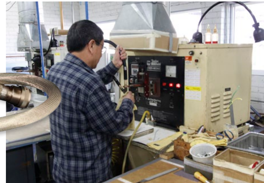
▼ Induction welding equipment and fixtures for fabrication of sealed metal-core conduit wire protection and routing assemblies
