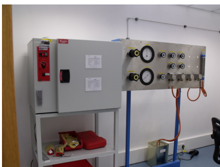
Pure air compatibility test equipment
