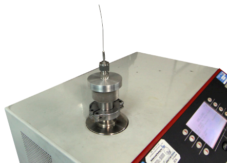
Gas tube helium leak test equipment
