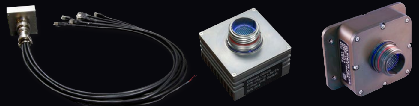
7-port Ethernet switch (shown with breakout test cable)
