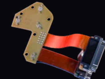
Stacked Micro-D I/O connectors with flex jumper to rigid PCB assembly
