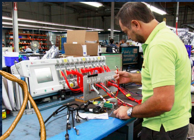
Continuity testing standard on all cable circuits
