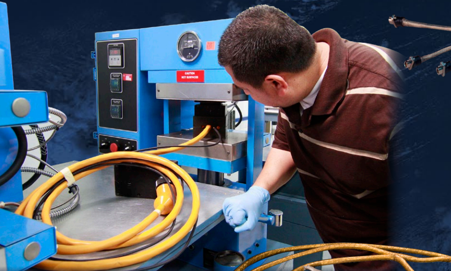
High-speed production overmolding
