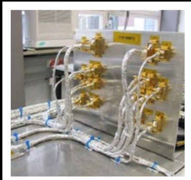
Turnkey satellite test harnesses and Electronic Ground Support Equipment racks
