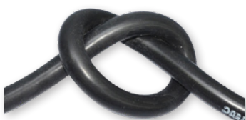
TurboFlex bend radius (Duraelectric jacketing) is 3X the outer diameter
