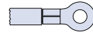
Small Ring for Attaching Receptacle Covers to a Panel with a Screw
